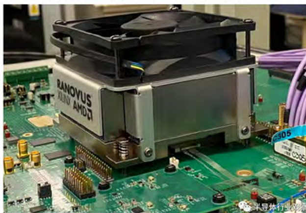
Figure 6.1: AMD Xilinx Versal ACAP co-packaged with Ranovus' Odin™ Analog-Drive CPO 2.0
