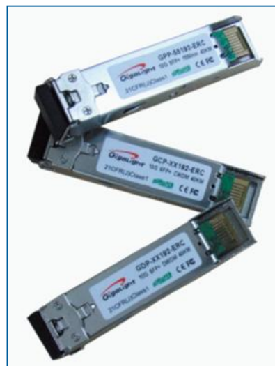
10G 40km SFP+光收发模块, for 1550nm, CWDM and DWDM
